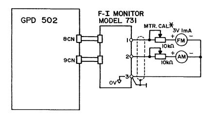
\* MTR. CAL can be omitted by setting of control constants Cn-24 and Cn-25. Otherwise, observe meter and calibrate for lmA full scale deflection.
