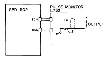
Figure 2. Interconnection Diagram For Pulse Monitor
