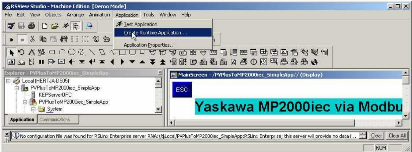
Figure 34: Compiling the HMI project
