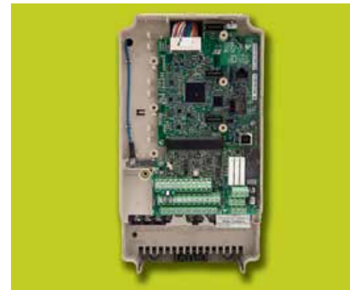
Easy Power & Control Terminal Access
