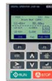
LCD Operator (all 1000 Series Drives)
