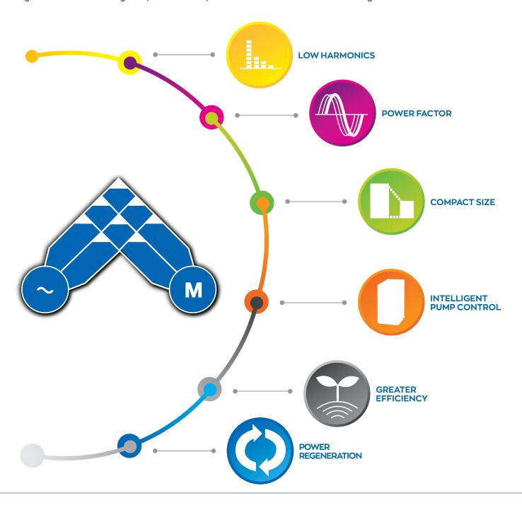
The U1000 iQpump's direct AC-to-AC power conversion is the most efficient IEEE 519 compliant solution on the market.
