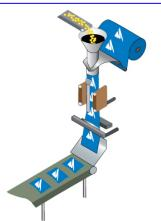
Many applications in **Assembly** or **Converting** involve feeding a product to a precise length either based on a pre-programmed distance, or to a registration mark. In many cases, the feeding mechanism consists of pinch rollers. In others, a clamp and push/pull method is used. Yaskawa's Feed-to-Length Solution can operate in either mode with either mechanism to provide precise product feeds with a minimal amount of programming.
