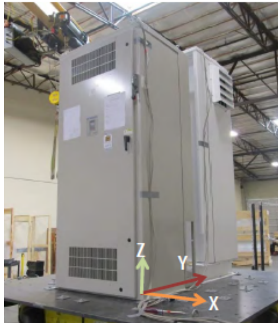
All units were filled with contents and maintained structural integrity and functionality
