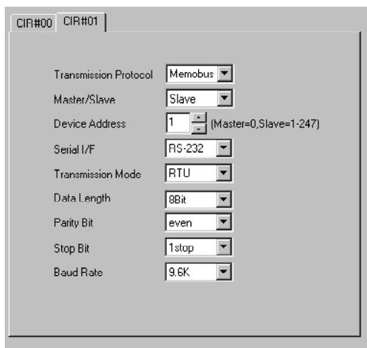
Figure 1.5 Setting Example for Module Configuration Definition Window (SLOT02)
