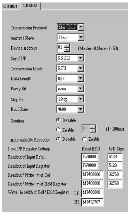
Figure 1.6 Setting Example for Module Configuration Definition Window (MP920)
