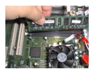
Ensure that the DIMM is fitted securely in the slot and that the latches to the left and right of the DIMM are fully upright. To remove the DIMM, the latches must be pressed down, which releases the DIMM from the slot. The DIMM can then be easily pulled out. DO NOT pull the DIMM without first pressing the latches. Then, close the CPU rack, plug the power cord into the CPU rack, and power ON. A memory count of the total RAM size then appears on the screen.
