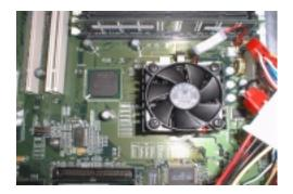
Follow the steps below to remove the CPU cooling fan.
