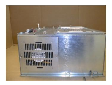
Figure 2.3: CPU Rack and Fan
