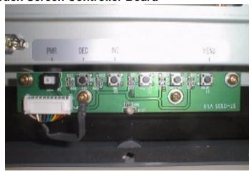
Remove the touch screen controller board by following the steps below.
