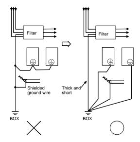
If a noise filter is located inside an enclosure, connect the noise filter ground wire and the ground wires from other devices inside to the ground plate of the enclosure first, then ground these wires.
