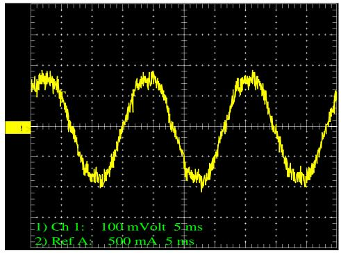
The field ground (FG) current of a machine. 60 Hz AC current is flowing in the FG wire. This may be caused by a ground fault somewhere in the building. This condition will cause nuisance tripping of the servo amplifier.
