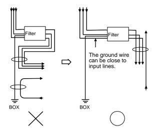
Connect the noise filter ground wire directly to the ground plate. Do not connect the noise filter ground wire to other ground wires.
