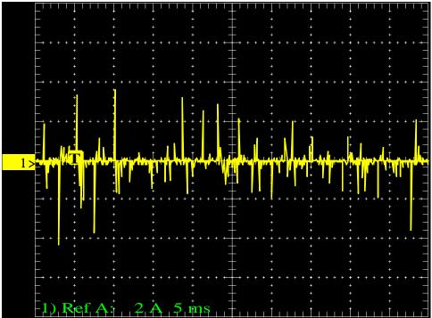
Normal FG current of a 400V Sigma II system at stand-still with Servo ON. This is the common mode current due to the switching of the IGBT's in the amplifier. Based on past experiences, the peak of the current pulses should be less than or equal to 2A during normal operation of a properly grounded servo system.
