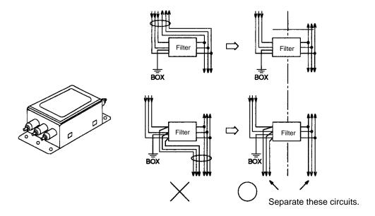
Isolate the noise filter ground wire from the output lines.
